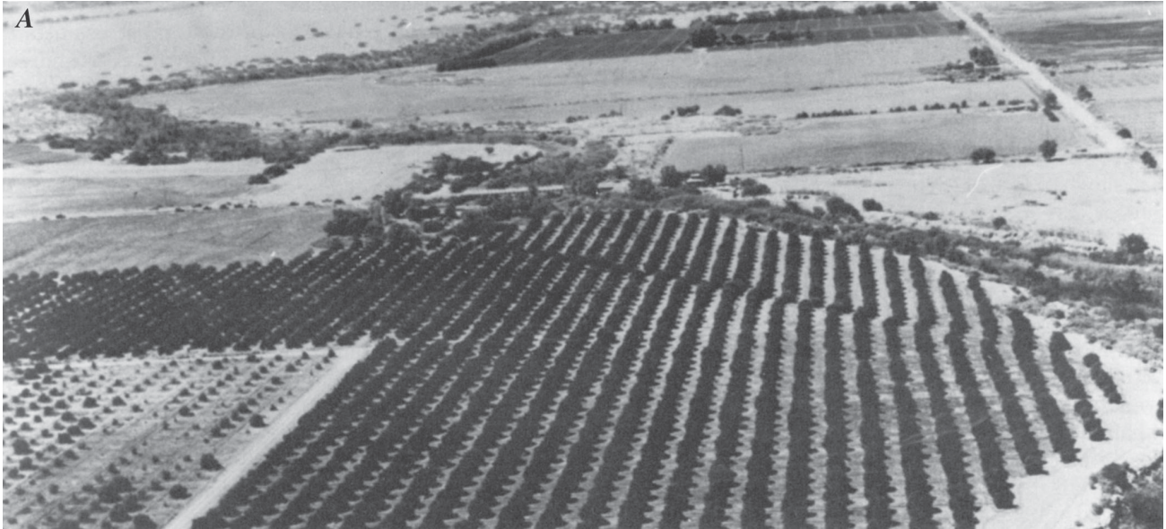
Figure 2.16. Two photos showing the effects of fault rupture. During an earthquake, the Earth's surface along a fault can be suddenly and permanently offset by many meters. Photo A shows the result of 6 meters of offset that occurred during the 1940 Imperial Valley earthquake in southern California. Photo B shows the crack left by 6 meters of offset that occurred near Point Reyes during the 1906 San Francisco earthquake. Imagine what would happen to anything built across the fault. (Photos from Wallace, R.E., ed., 1990, The San Andreas Fault System, California : U.S. Geological Survey Professional Paper 1515, p. 163.)
