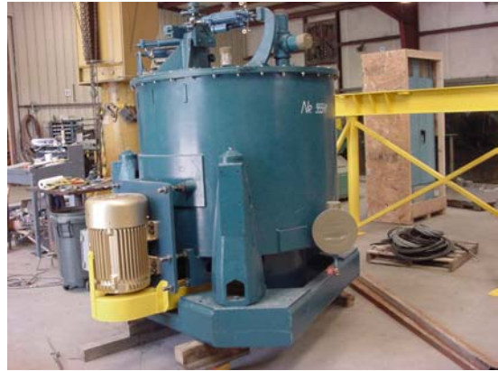
The Triton TS-5000 separator, the first of three solids separation technologies to be evaluated through the Water Quality Protection Center for the treatment of flushed swine waste.
