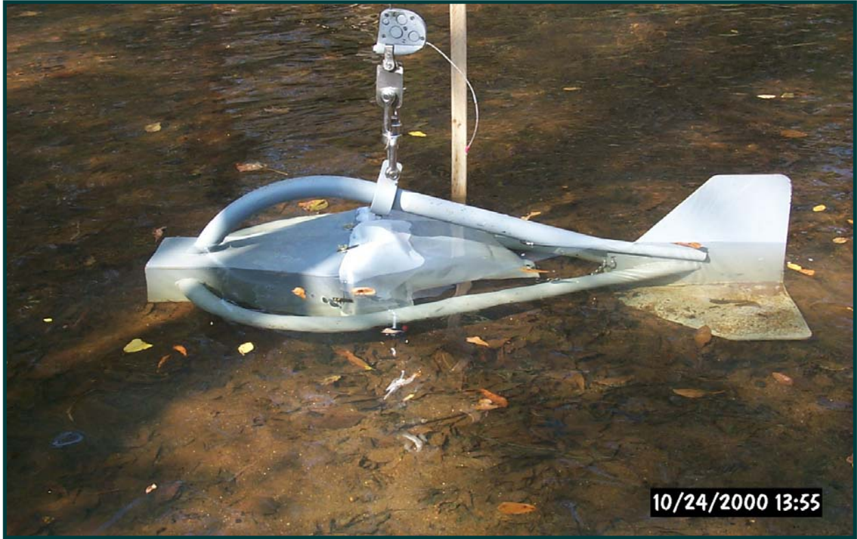
Figure 18: 6-inch Helley-Smith Bedload Sampler
