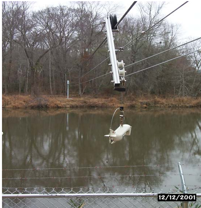
Figure 19: Depth Integrated Sampler
