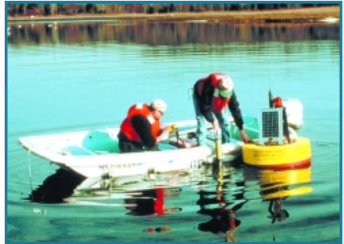
Figure 4.13. Inshore/harbor monitoring buoy being deployed from a small work boat
