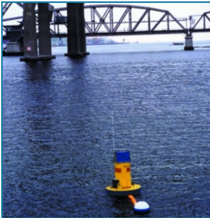
Figure 4.7. MYSound inshore buoy monitoring station in the Thames River, New London, CT
