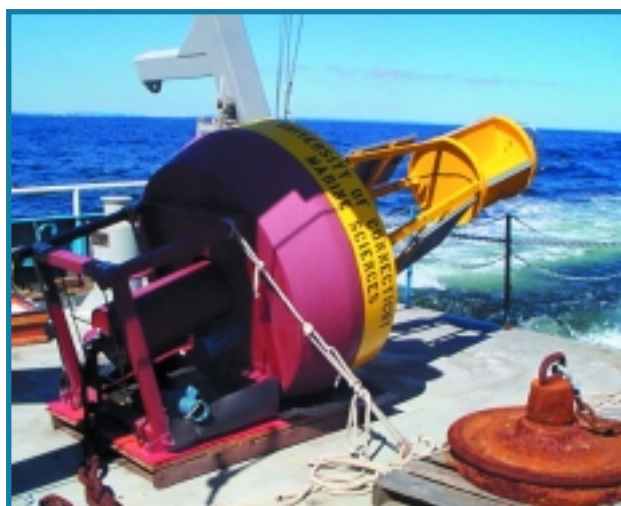
Figure 4.12. Buoy and mooring equipment for an offshore monitoring station arrayed on deck prior to deployment
