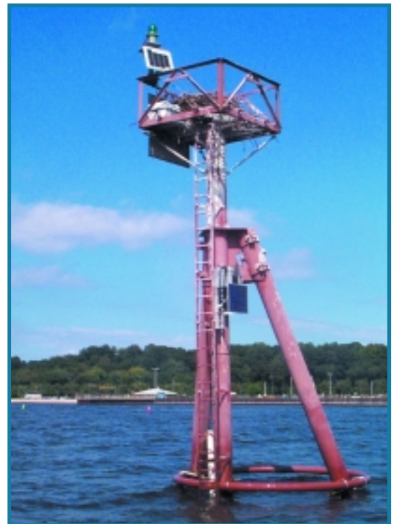
Figure 4.8. Hempstead Harbor monitoring station deployed on a Coast Guard Aid to Navigation
