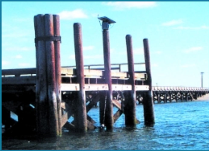
Figure 4.9. The Bridgeport Harbor monitoring station deployed from a pier. Note solar panels on pier.
