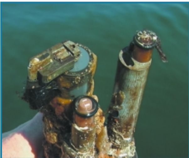
Figure 4.14. Biofouling on a YSI sensor package
