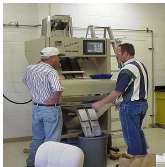
High speed sorter used to improve grain quality.
