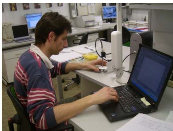
Using ERU NIR technology to scan mosquitoes for the International Atomic Energy Agency.
