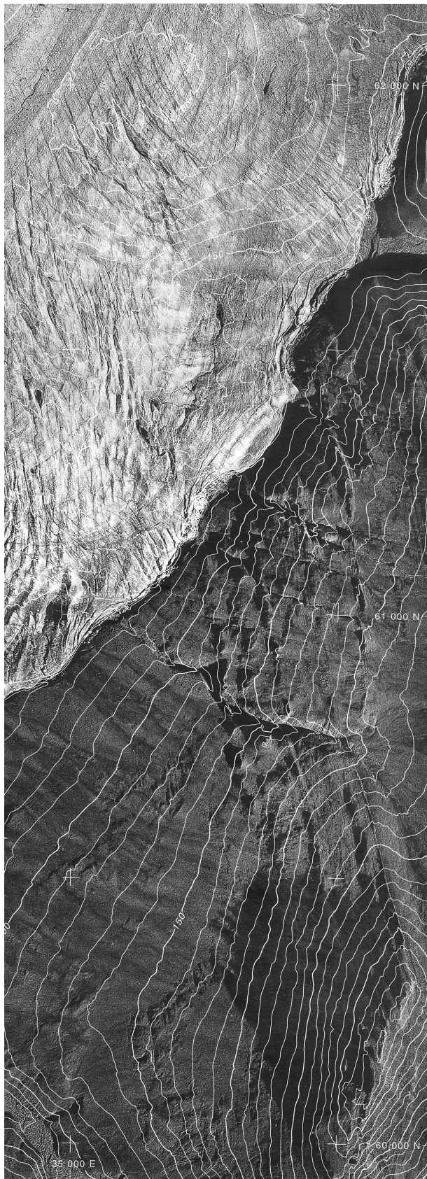
Figure 6. —Orthophoto map of the Thompson Glacier termini, Axel Heiberg Island, Nunavut; reduced from the original scale of 1:5,000; contour interval 10 m. Map based on 1977 aerial
