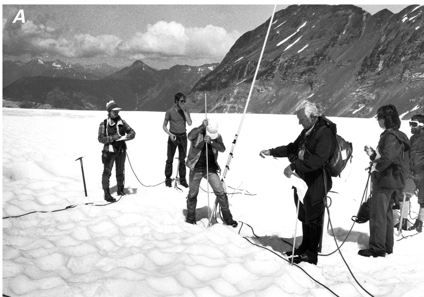
Figure 10. —Photographs of the Place Glacier, Coast Mountains, British Columbia. A , Dr. Gunnar Østrem and members of the 1980 Field Glaciology Course making mass-balance measurements on Place Glacier. In 1965, as part of a major expansion of glaciological studies during the International Hydrological Decade, Place Glacier was selected to be part of an east-west transect of glaciers to be monitored in western Canada. The mass-balance measurements begun here in 1965 have continued to the present day. B , Terminus of the Place Glacier and its proglacial lake in October 1975. Photograph by Oleg Mokievsky-Zubok, National Hydrology Research Institute. (Glacier 62 in table 1) [INTS Map: 092J07]
