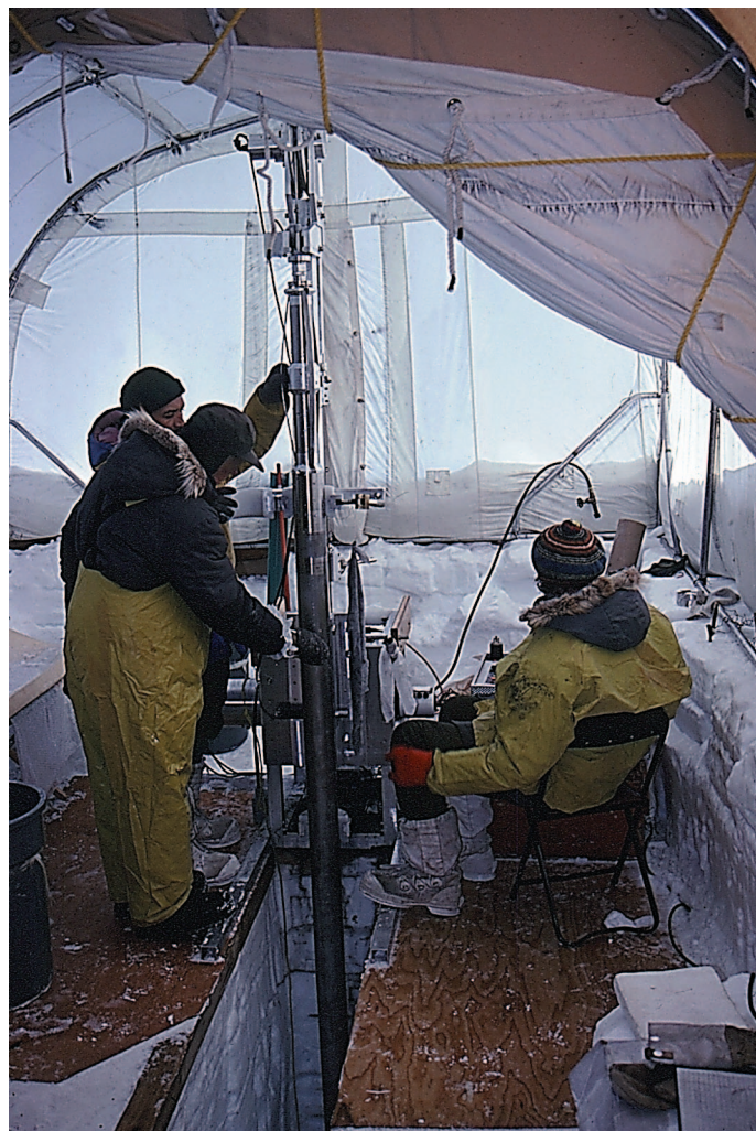
Figure 17. —Photograph of the electro-mechanical ice-core drill being lowered into the borehole on top of the Devon Ice Cap in April 1998. The drill was used in a partially fluid-filled borehole to minimize core fracturing. Lamp oil was used as a fluid and is filtered and re-used during drilling operations. On ice caps where the ice at the top of the flow line is often about 300-m thick, core fracturing usually begins at a depth of about 150 m and consists of microfractures that obscure the stratigraphy. Geological Survey of Canada personnel working in the shelter tent are as follows: D.A. Fisher is at the control box on the right; C. Zdanovicz has his hand on the torque springs on the left; and R. M. Koerner is in the left foreground. The torque springs prevent the outer sonde casing and the cable from turning in the borehole. Geological Survey of Canada photograph.
