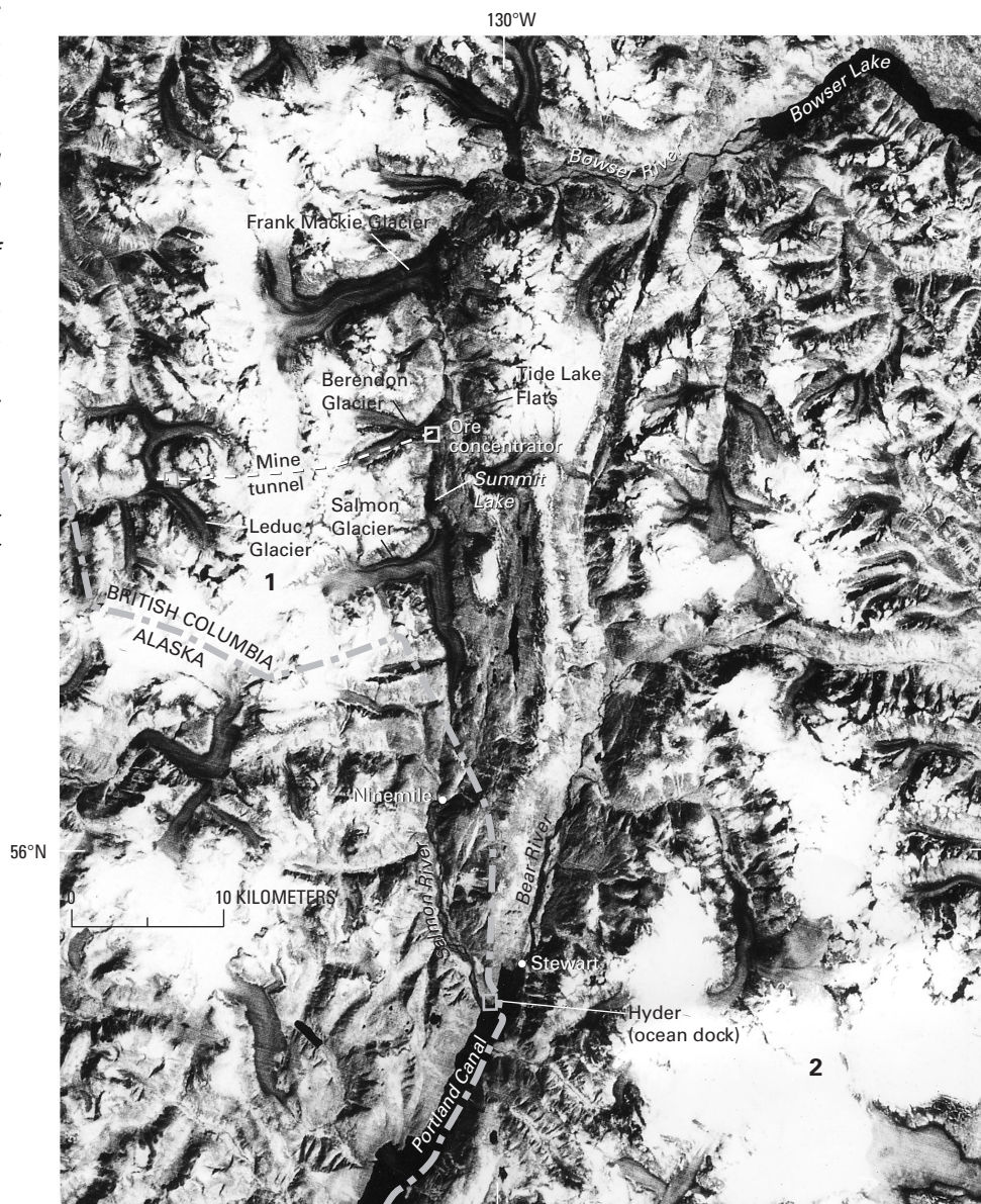
Figure 2. — Annotated Landsat MSS image of part of the Coast Mountains near Stewart, British Columbia, and the Granduc mining development. Copper ore is transported through an 18-km tunnel from a mine (shown by a small box) near Leduc Glacier east to a concentrator at the terminus of Berendon Glacier, then by truck to an ocean dock near Stewart. Annotations: 1, the Frank Mackie highland glacier complex; 2, Cambria Snowfield. Landsat image (21288–18435, band 7; 2 August 1978; Path 58, Row 21) is from the EROS Data Center, Sioux Falls, S. Dak. Map references: Leduc Glacier sheet 104B/1 and 104B/2, 1:50,000; Iskut River sheet 104B, 1:250,000.
