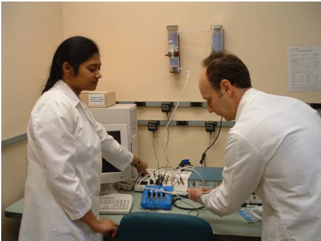
Dr. George Yocum and Anitha Chirumamilla changing a column on the Sable Systems respirometer used in oxygen/carbon dioxide respiration studies of larval sugarbeet root maggots.
