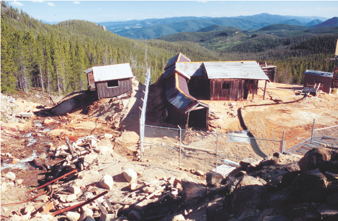
Figure 7. Crystal mine, June 1997. Acidic discharge drains from adit (out of view near lower right of photograph) to Uncle Sam Gulch on far left. Photograph by D.A. Nimick.
