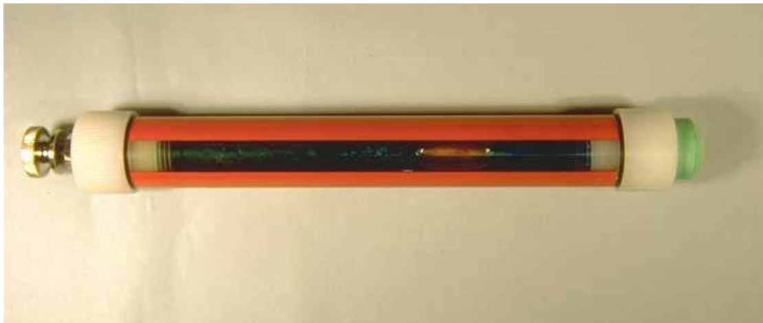
Figure VIII-7 Reference Electrode – A saturated copper-copper sulfate half-cell.
