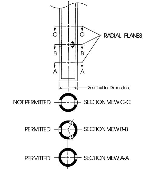
Figure B114-2 SAMPLE PROBE AND TYPICAL HOLE SPACING
