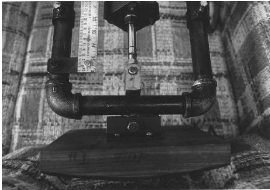
Figure 16. A clevis type bracket attached to the rear of the load head provides a means of attaching the load head to the crossbar of the internal load frame. Position of the cross hole in this bracket controls the amount of movement of the load head both up and down and side to side. A male rod end to which the load head is attached passes through the cross bar of the internal load frame and threads into the body of a clevis.
