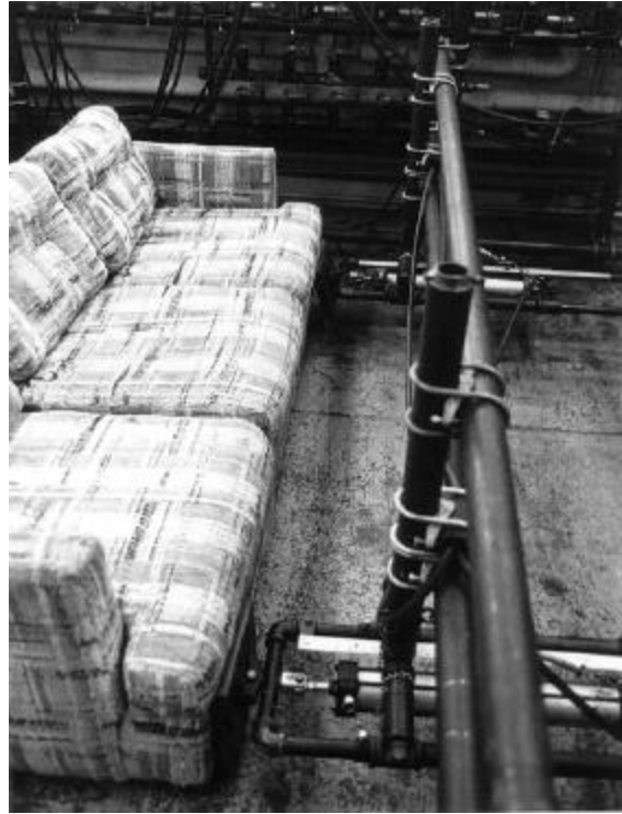
Figure 23a. Arrangement of a sofa in the main testing machine frame for carrying out the front to back load test for legs. A length of 3/4 inch diameter pipe placed behind the back legs of the sofa prevents the sofa from sliding backwards during the test and also provides the reaction forces required to test the legs.
