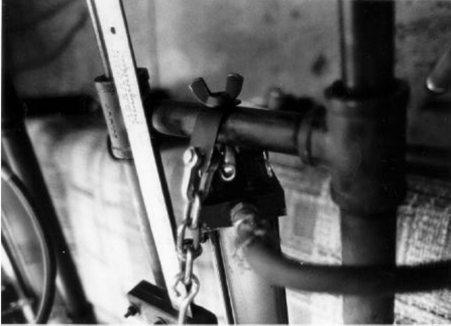
Figure 14. The clevis bracket attached to the rear end of the air cylinder provides a means of attaching the body of the cylinder to the crossbar of the external load frame. A strap which is bolted to the crossbar by means of the rod end body and nut provides a point of attachment for a spring/turnbuckle/chain linkage which controls the angle of inclination of the test load frame.
