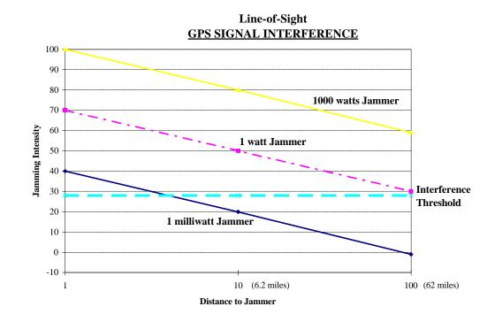
The horizontal axis represents the distance between the jammer and the typical Global Positioning System receiver in kilometers. The vertical axis represents the jammer interference to the Global Positioning System signal in decibels (dB) or the jamming intensity. The three diagonal parallel lines represent three jamming devices with different effective power measured in watts and milliwatts.
