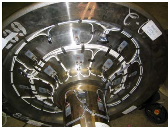
Figure 7. Back of instrumented wheelset, in the shop with cover off (note strain gauges and connecting wires)
