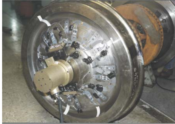
Figure 8. Outside face of instrumented wheelset, in the shop with cover off (note strain gauges)
