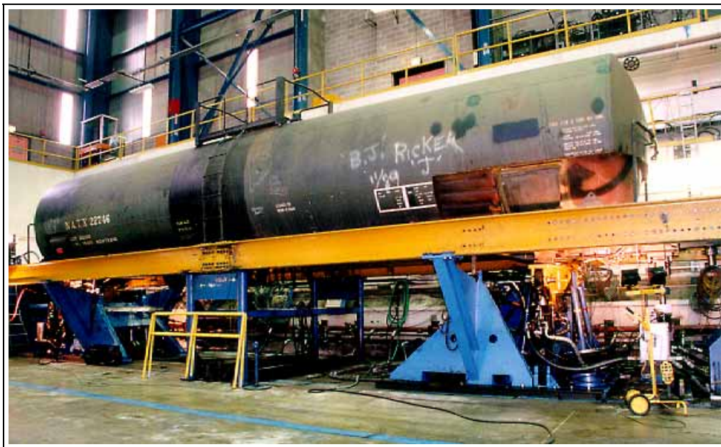
Figure 6. Test Car NATX 22746 on Simuloader
