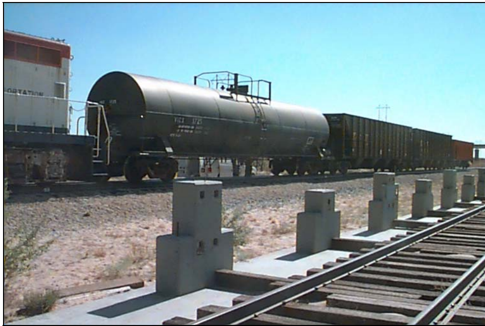
Figure 1. VICX 1725 Tank Car Setup for Impact Test
