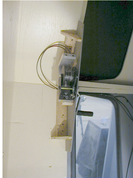
Figure 60. Winch installed overhead, oriented in rollover position
