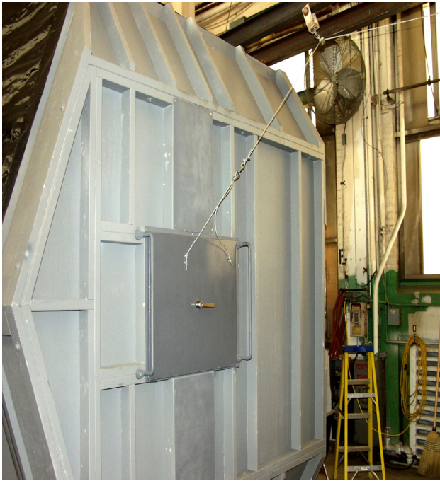
Figure 27. Hatch is attached to a tether line
