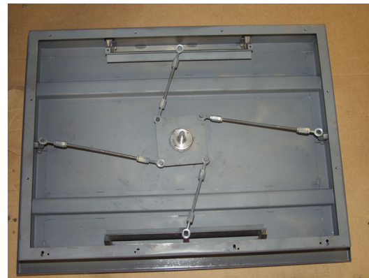
Figure 13. Latching mechanism in the open position
