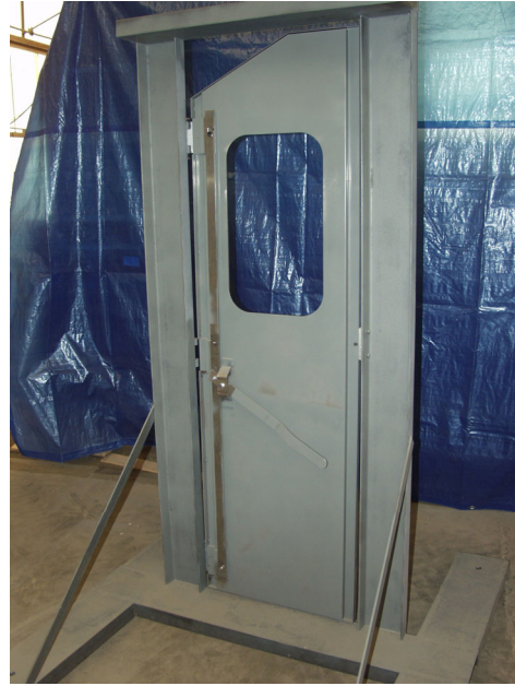
Figure 75. Final position of the hinge release handle after actuation
