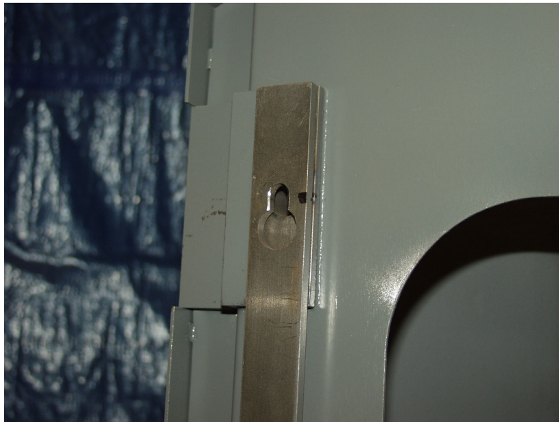
Figure 76. Interior closeup view of the released fastener nut
