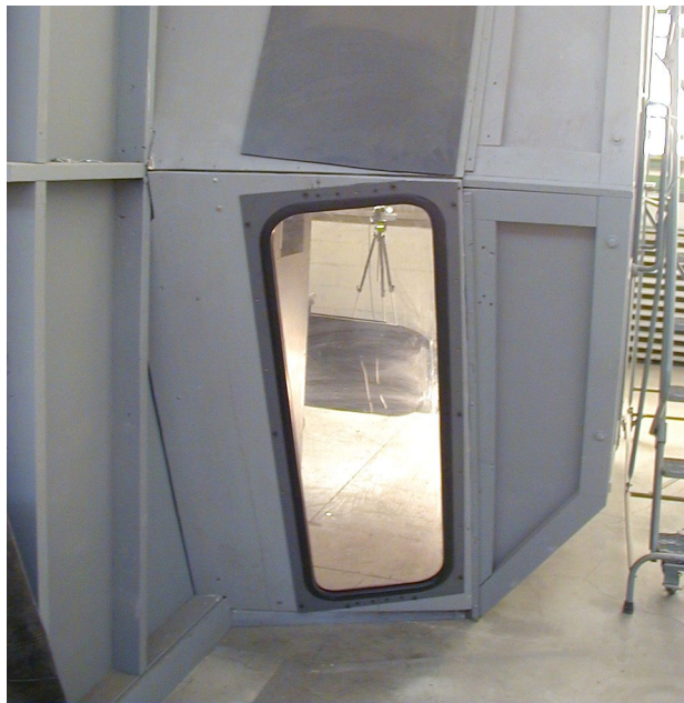
Figure 56. Exterior view of windshield frame mounted in mockup locomotive
