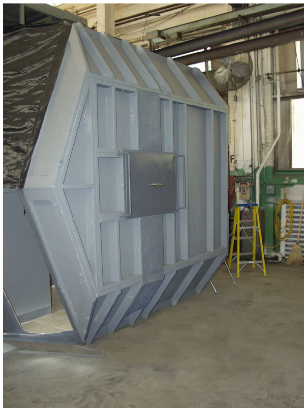
Figure 25. Mockup of toppled locomotive cab with egress system
