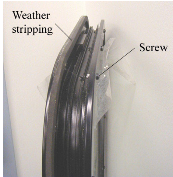
Figure 34. Closeup view of GE windshield assembly
