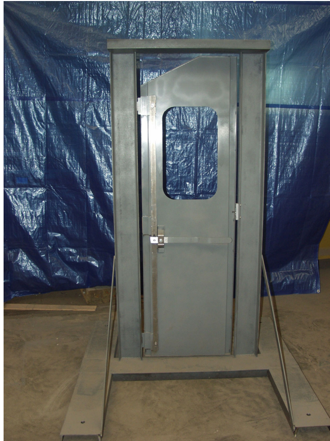
Figure 72. Interior view of the rear door with hinge release handle in assembled condition
