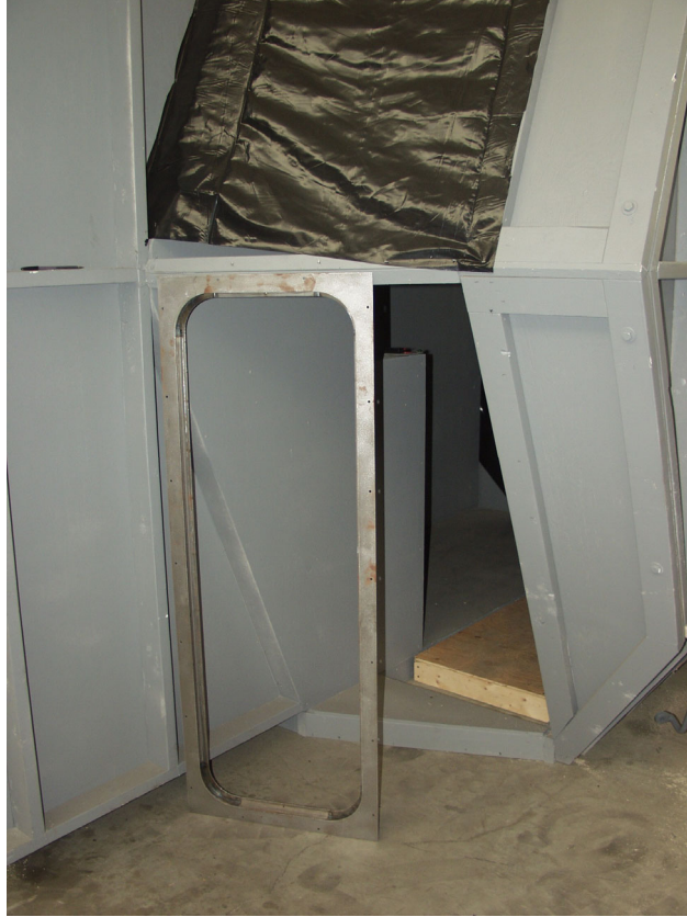
Figure 55. Steel mockup windshield frame installed in mockup
