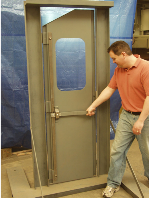
Figure 74. Interior view of the door showing the actuation of hinge release handle
