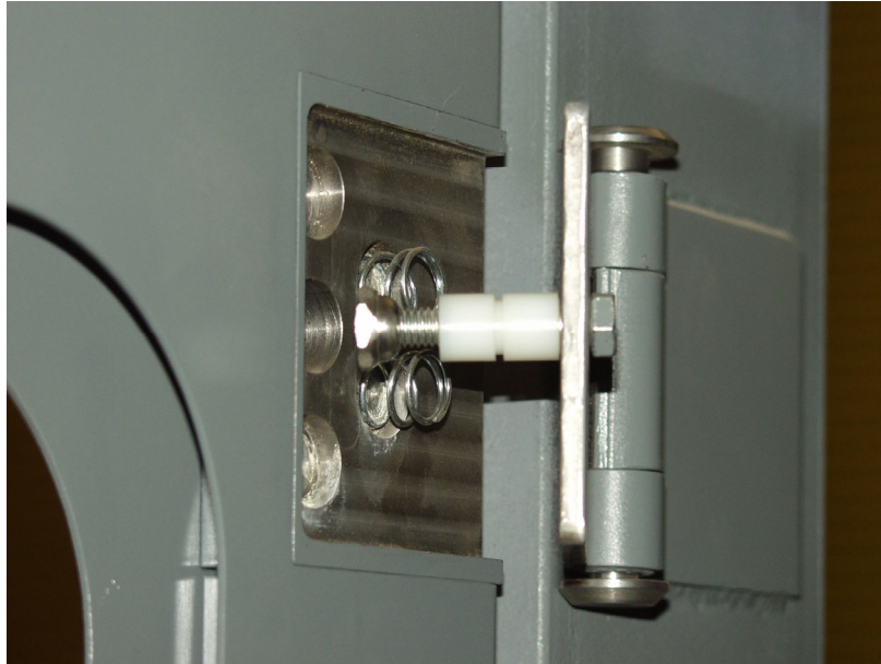
Figure 77. Exterior view of the fastener bolt and hinge leaf released from the hinge support block
