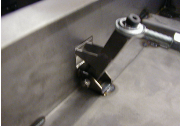
Figure 17. Latch cam in the open position, interior
