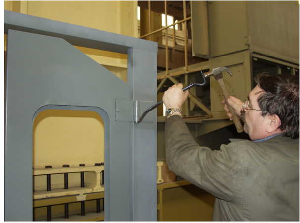
Figure 80. Removal of the hinge pin before separation of the rear door
