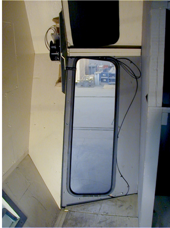
Figure 57. Interior view of windshield frame mounted in mockup locomotive
