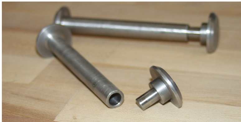
Figure 69. Hinge pins and the interference fit small pin-inserts with cap
