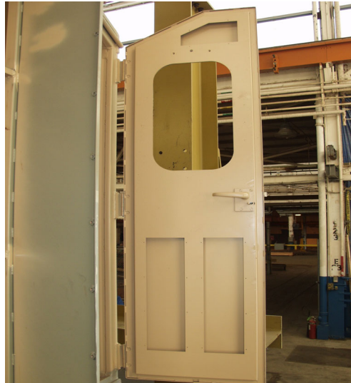
Figure 63. Interior view of the existing locomotive rear door at a test facility
