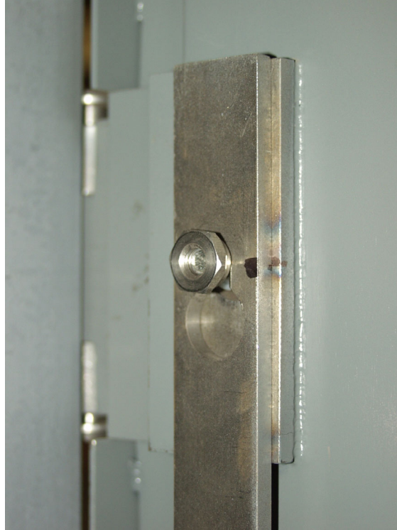
Figure 73. Closeup view of an acorn nut assembled on the narrow slot of the key-hole in the sliding bar
