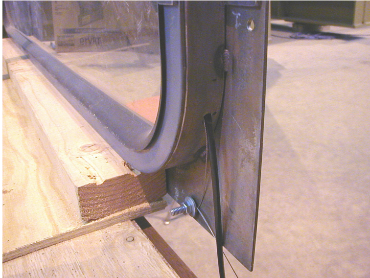
Figure 52. Wire sleeve for cutting wire
