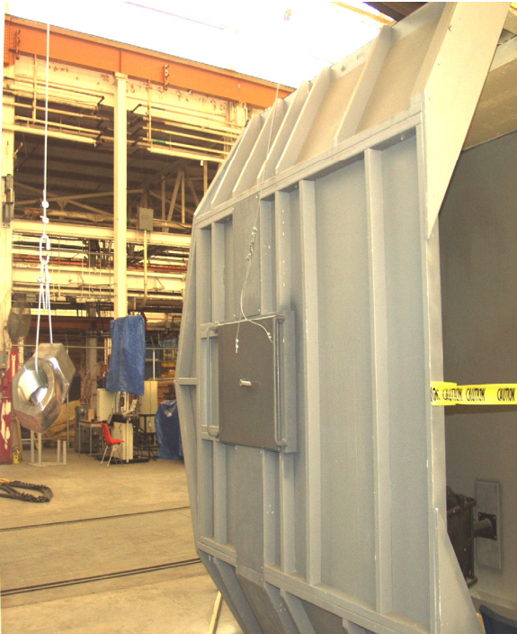
Figure 30. Counter weights allow hatch to settle gently
