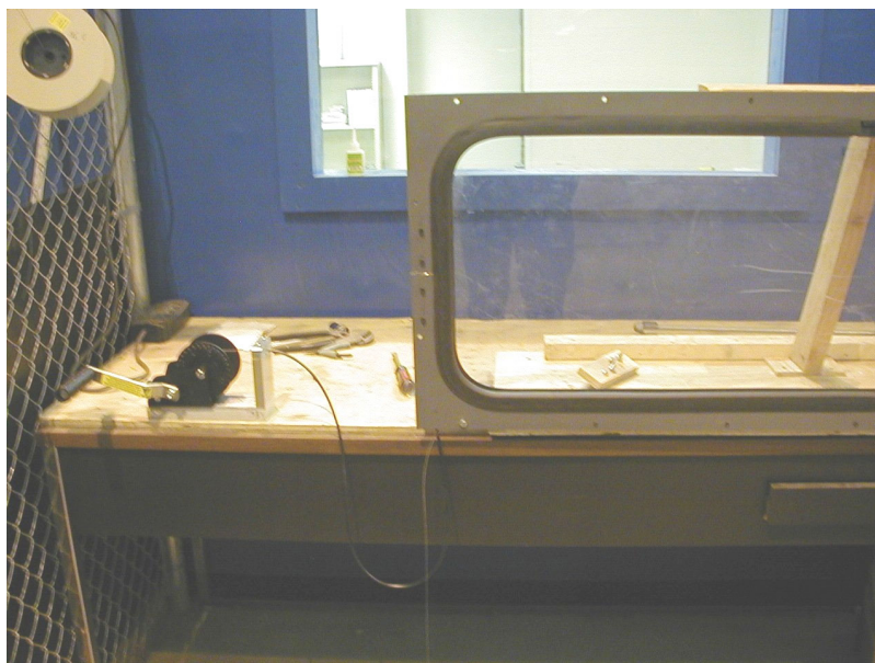
Figure 51. Wire sleeve from windshield frame to winch
