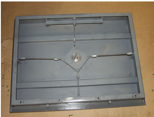
Figure 12. Latching mechanism near the closed position
