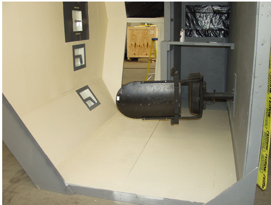
Figure 26. Interior view of cab mockup with hatch system
