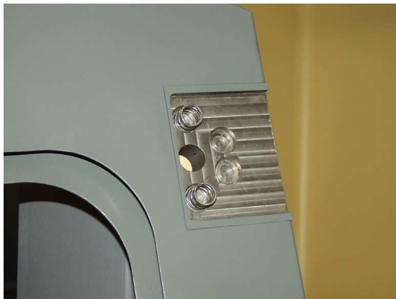
Figure 78. Closeup exterior view of a hinge support block after detachment of the hinge leaf
