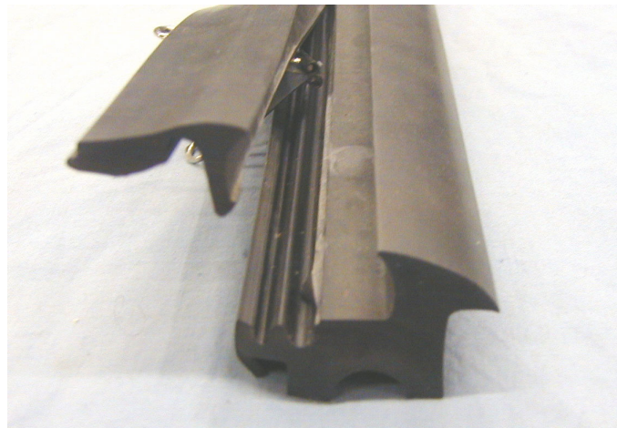
Figure 61. Gasket after being severed by wire
