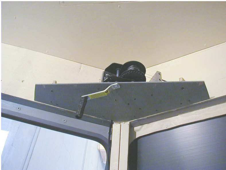
Figure 59. Winch located in overhead console of mockup locomotive
