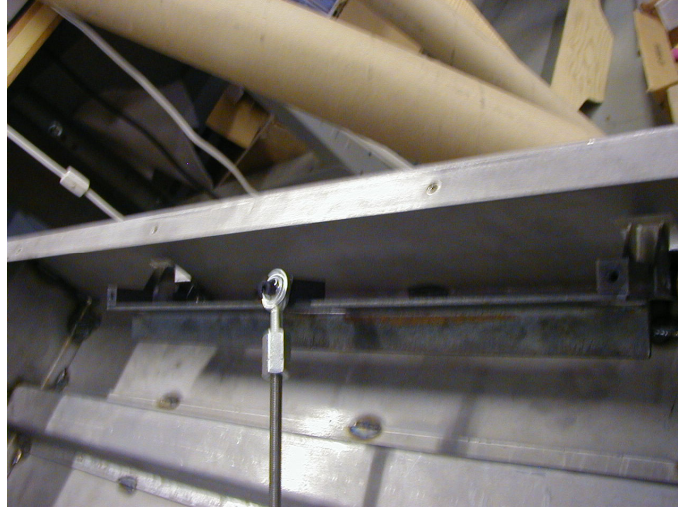
Figure 14. Side latch cams and latching bar
