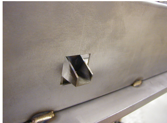
Figure 16. Latch cam in the latched condition, exterior
