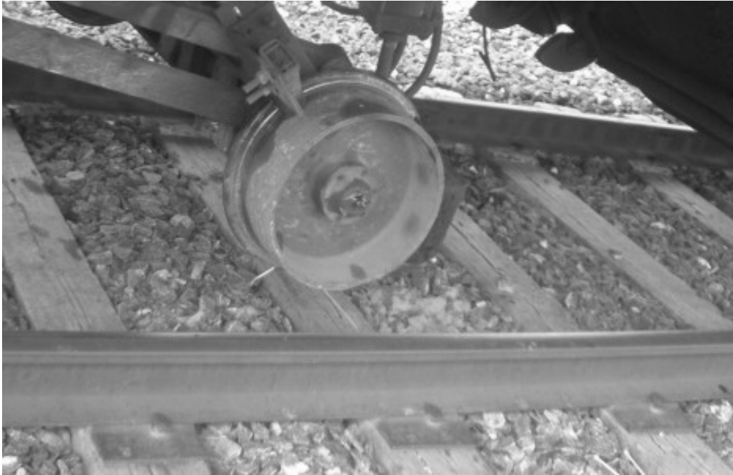
Figure 5. FRA's GRMS Unloaded Gage Measuring Axle Assembly in the Retracted Position
