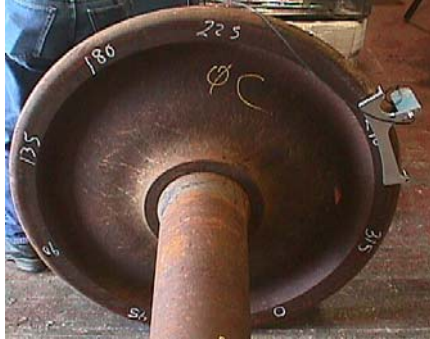
Wheel #14073 a tread damaged wheel at Progress Wheel Shop
