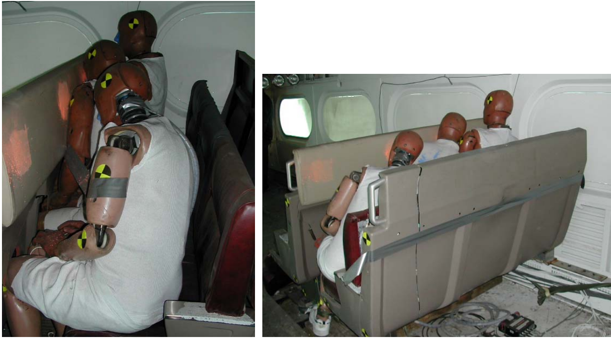
Figure 36. Experiment No. 1-1 – Occupants Remain Compartmentalized
