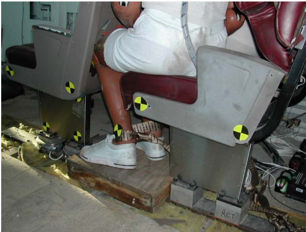
Figure 41. Experiment No. 2-2 - Post-Test Close-Up View Shows No Seat Frame Deformation
