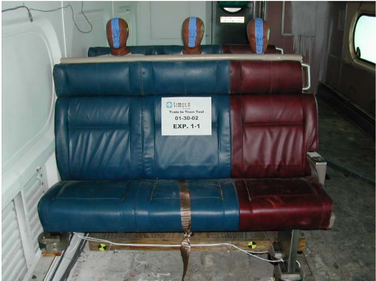
Figure 18. Pre-Test Photo of Experiment No. 1-1, Row-to-Row M-Style Seats
