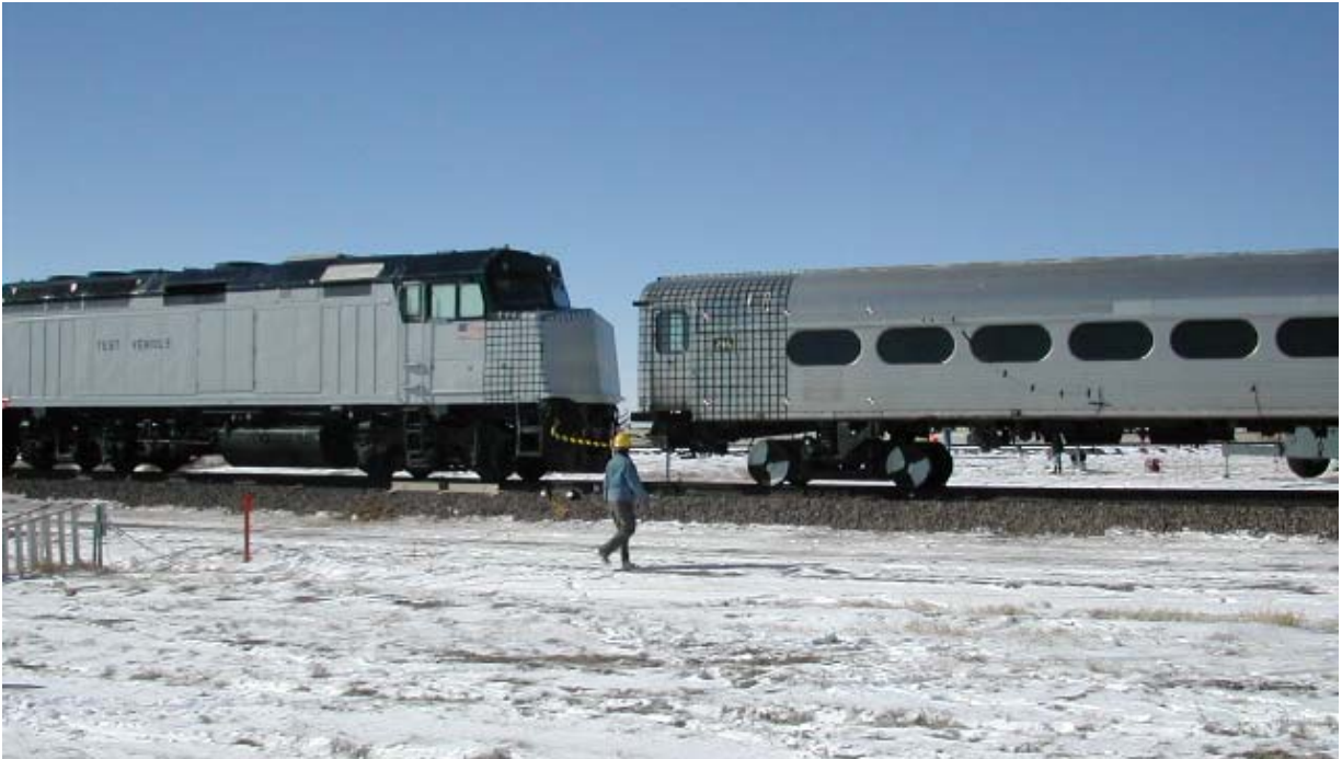
Figure 10. Pre-Test Impact Site - Leading Cab Car and Stationary Locomotive
