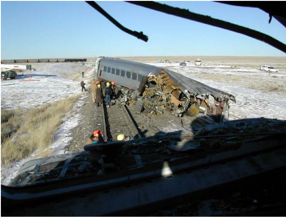
Figure 32. Post-Test View of Leading Cab Car, Right Side, Through the Broken Windshield of the Impacted Locomotive
