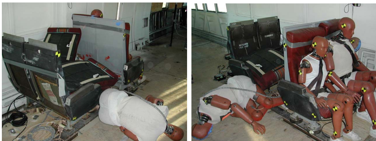
Figure 37. Experiment No. 2-1 - Front and Aft Views, Post-Test
