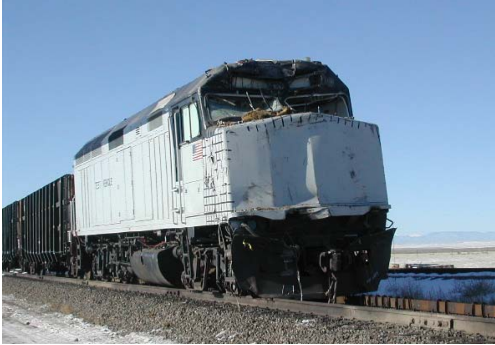
Figure 31. Post-Test View of the Impacted Locomotive
