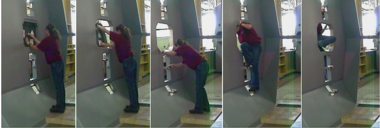
Figure 36. Egress of 50 th Percentile Female Subject, Interior View
