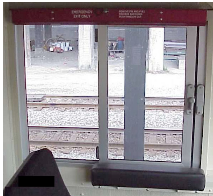
Figure 5. Removable Side Window for F59-PHI Locomotive by R. E. Jackson, Co.
