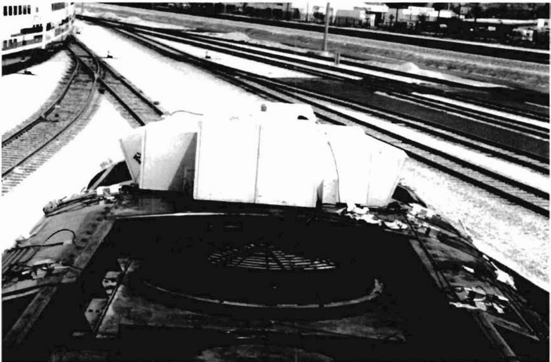
(b) Microphones Taped to the Locomotive Hood
