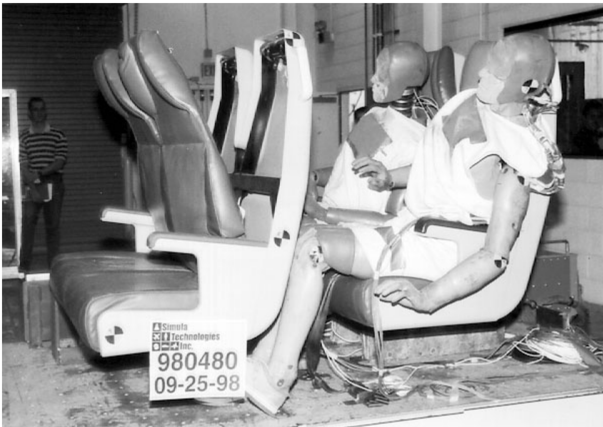
Figure 23. C-3 Seat Post-test - Type 1 Test (98-0480)
