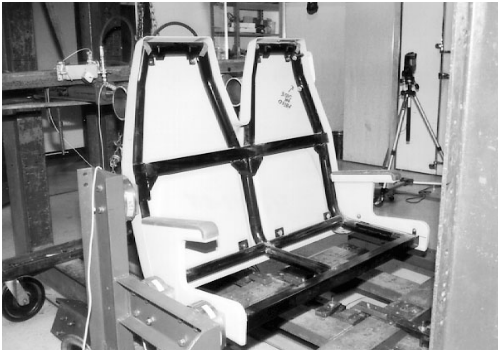
Figure 2. C-3 Commuter Seat Setup for Static Testing in the Test Frame
