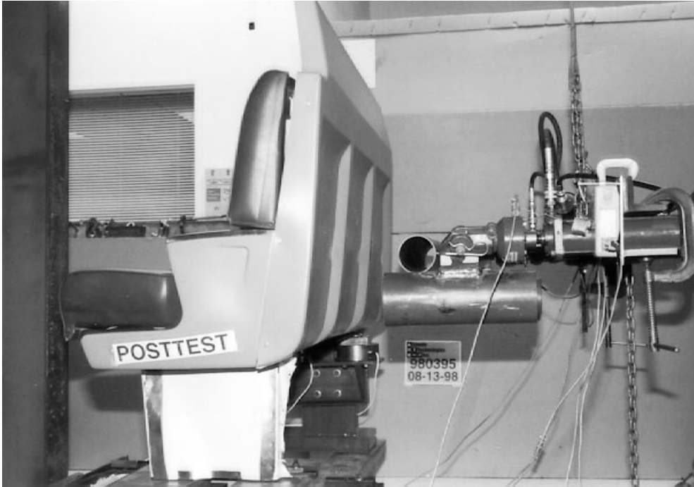
Figure 16. M-Style Lower (Post-test) - Pedestal Attachment Buckled and Seat Cushions Detached
