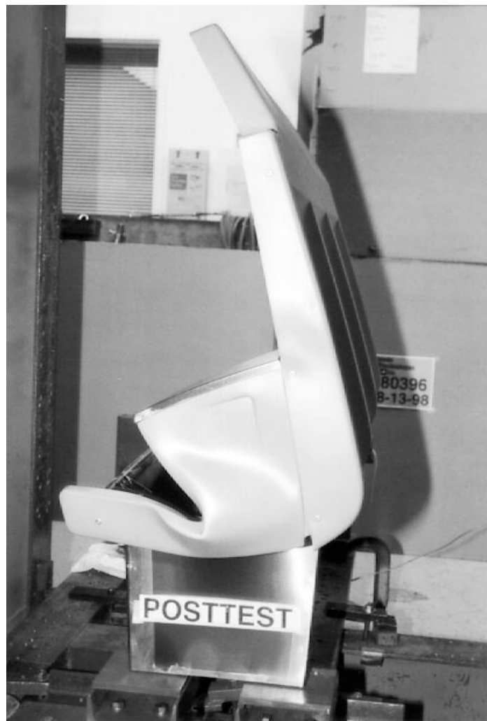
Figure 14. M-Style Upper (Post-test) - Seat Rotated Forward and Plastic Shroud Buckled at Armrest
