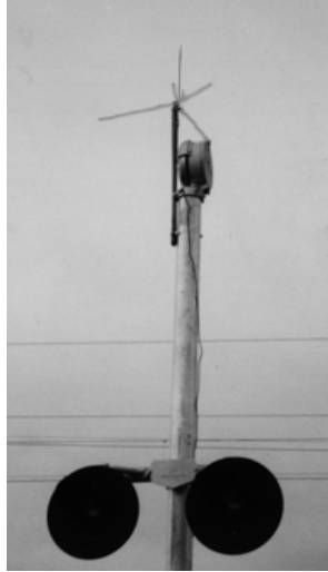
Figure 3-6. SmartStops Crossing Transceiver Antenna
