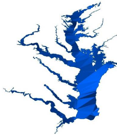
Figure 3-2: an exaggerated 3D view of the MHHW sea level surface within the Chesapeake Bay area.
