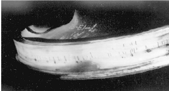
Figure 2. Thermal cracks on commuter wheel tread.
