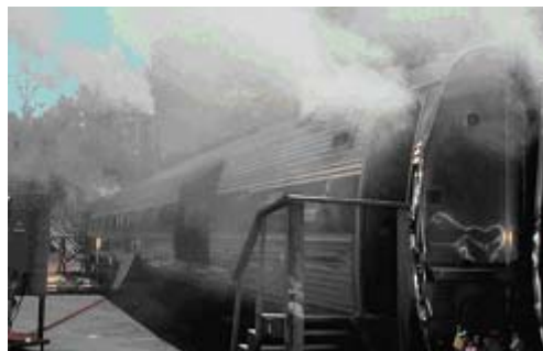
Figure 1. Full-scale fire test
