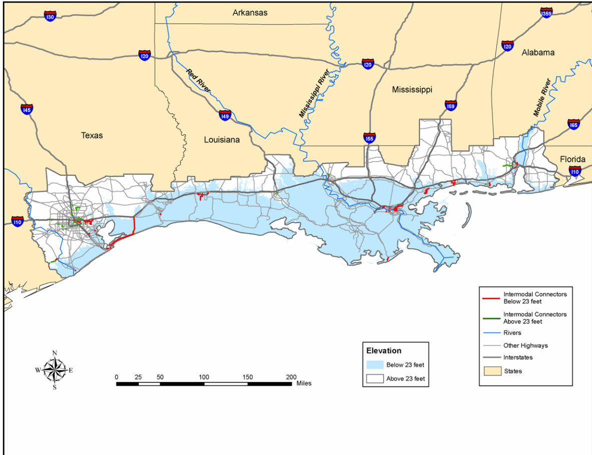
Figure 4.7 National Highway System (NHS) intermodal connectors at risk from storm surge at elevations currently below 7.0 m (23 ft). (Source: Cambridge Systematics analysis of U.S. DOT data)
