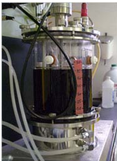
Kevin Moloney for The New York Times Chim Chin, a researcher at PureVision Technology, works with equipment that distills ethanol and leaves lignin as a byproduct.
