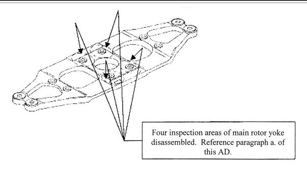
Figure 3. Main Rotor Yoke Inspection Areas
