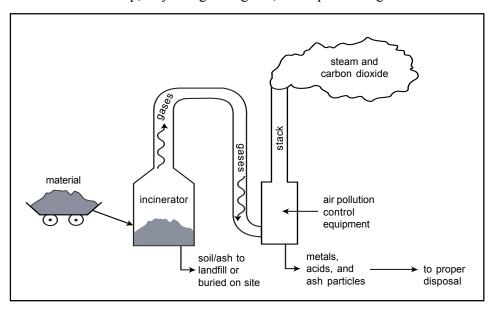
further. The gases become so hot they break down into smaller components that combine with oxygen to form less harmful gases and steam.
