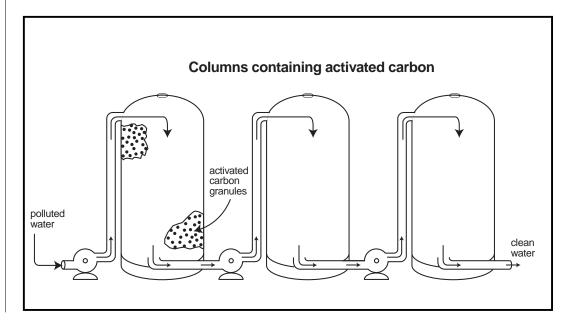
of the granules. The water or air that exits the column is cleaner than the water or air that entered it. If the water or air isn't clean enough, it is pumped into another column or cleaned using another method.
