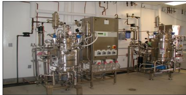
Fermentor used for mass production of biological control agents
