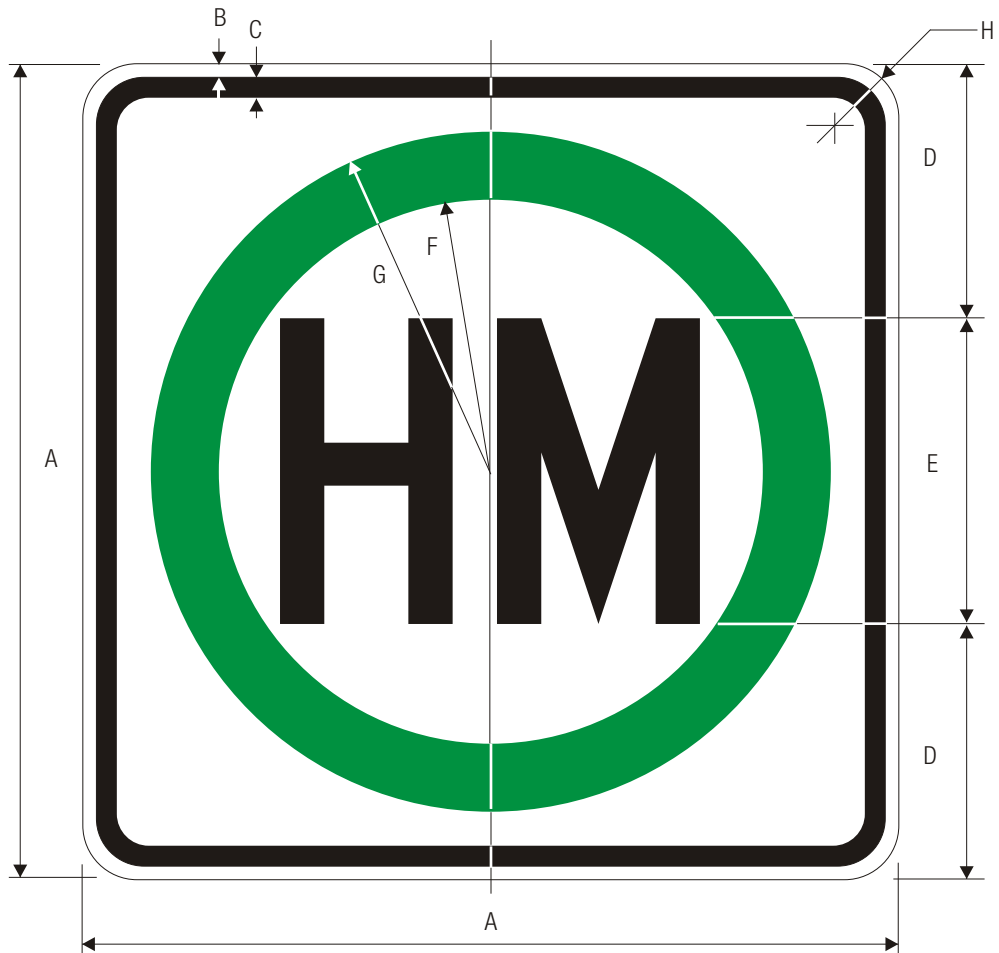
R14-2 HAZARDOUS MATERIAL
