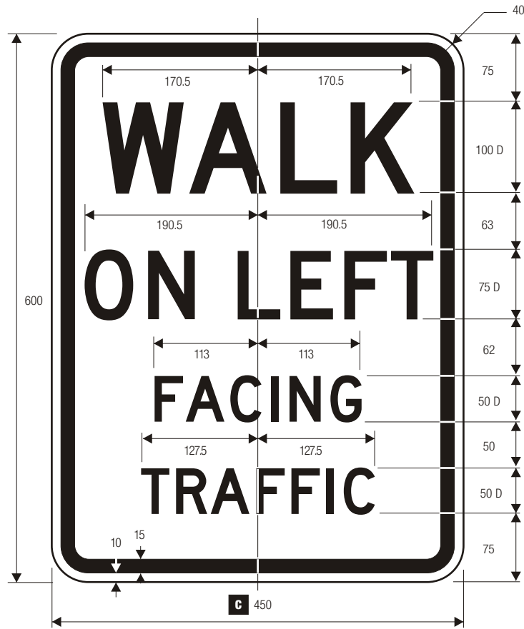
R9-1 WALK ON LEFT FACING TRAFFIC
