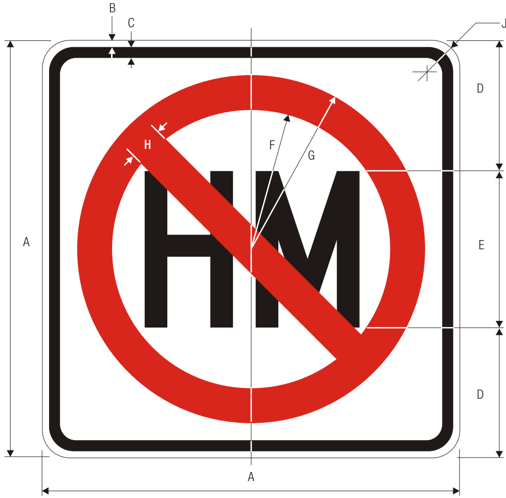
R14-3 HAZARDOUS MATERIAL
