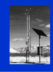
Road Weather Information Systems provide data on air and pavement temperatures, precipitation, and the amount of deicing chemicals on the pavement.
