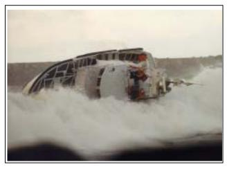
47-Foot Motor Lifeboat Rolling Over in Heavy Surf
