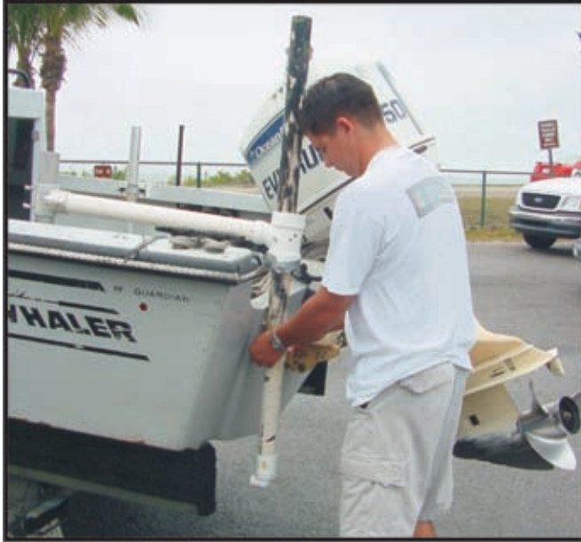
Figure 9. Flow-through chamber, for salinity survey, mounted to the transom of the boat.
