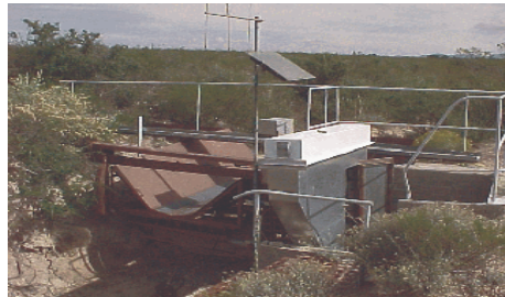
"Santa Rita" flume with traversing slot sediment sampler
