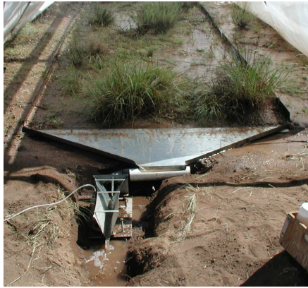
Plot scale rainfall simulator sediment yield experiment.
