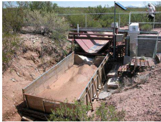
Santa Rita runoff measuring flume with traversing slot sediment sampler showing pit trap filled with sediment after a flow.
