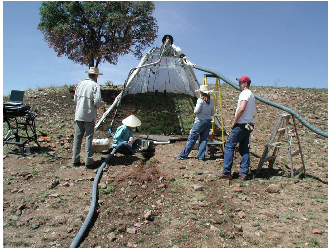
Rainfall simulation with the WGRS on a grassland site
