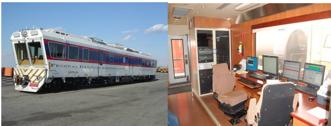
The FRA T-19 track geometry inspection vehicle (left) and the interior of the T-20 vehicle (right).
