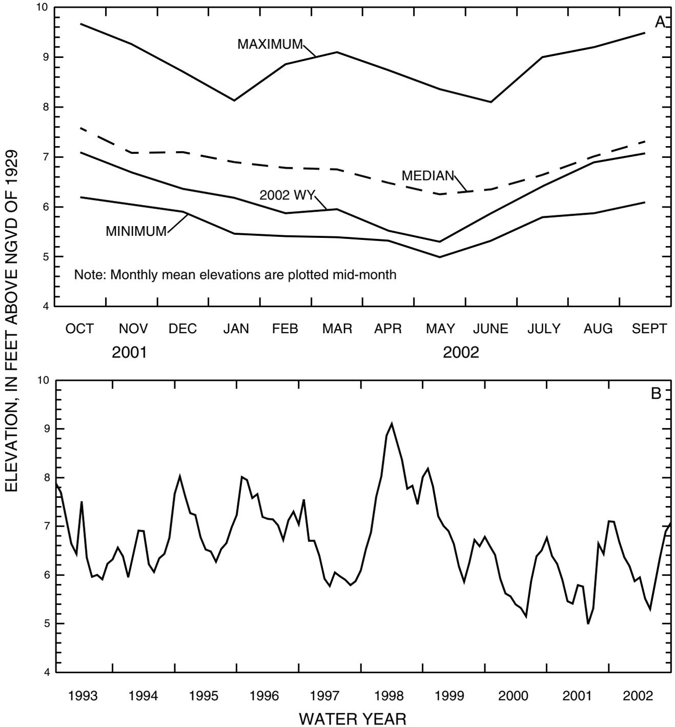
Figure 3.--Chassahowitzka well 1 near Chassahowitzka, Upper Floridan aquifer, (A) 2002 monthly mean elevation compared to the maximum, median, and minimum monthly mean elevation for the period of record, and (B) the monthly mean elevation for the period 1993-2002
