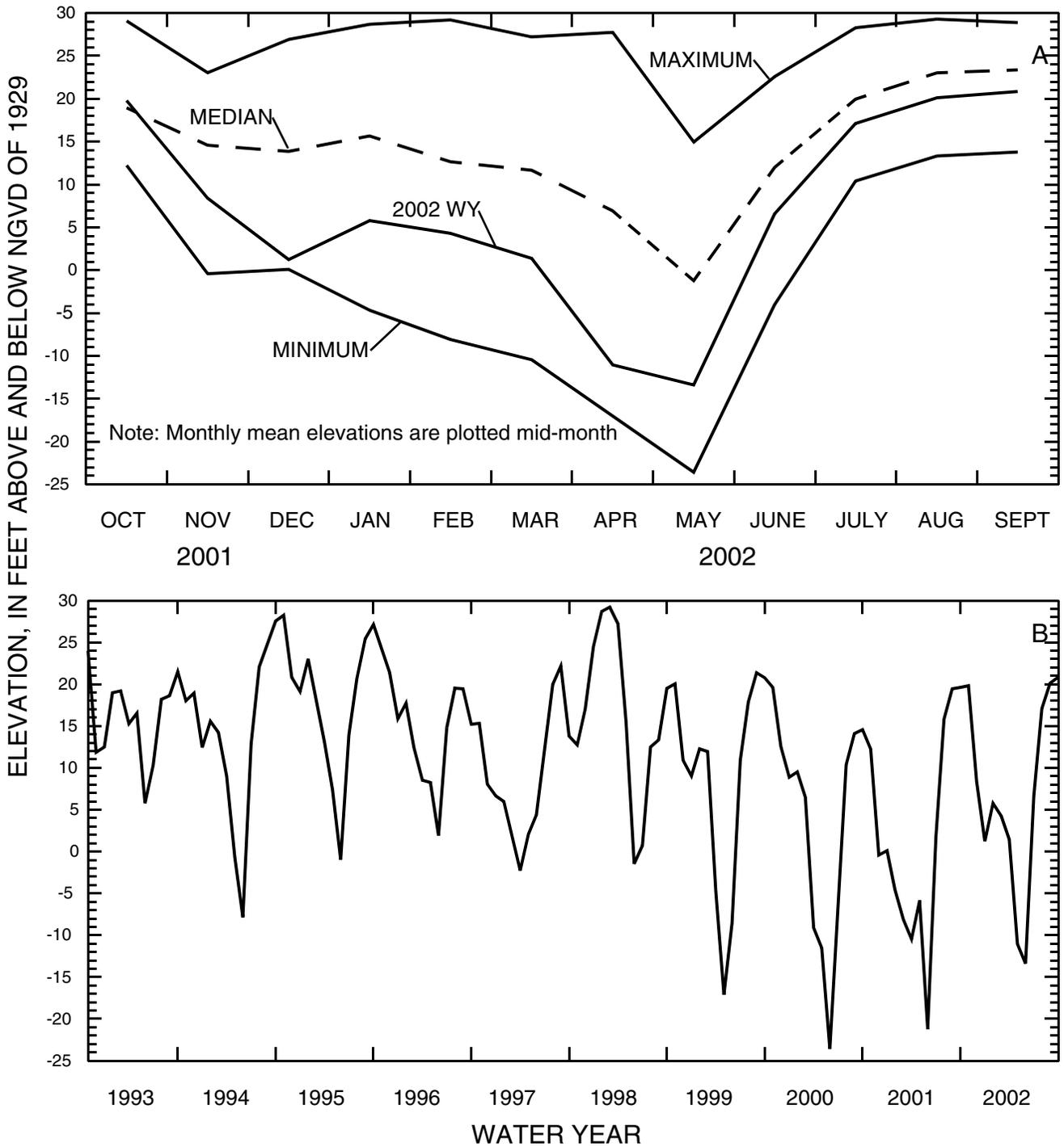
Figure 6.--Kibler deep well 26B near Bethany, Upper Floridan aquifer, (A) 2002 monthly mean elevation compared to the maximum, median, and minimum monthly mean elevation for the period of record, and (B) the monthly mean elevation for the period 1993-2002.
