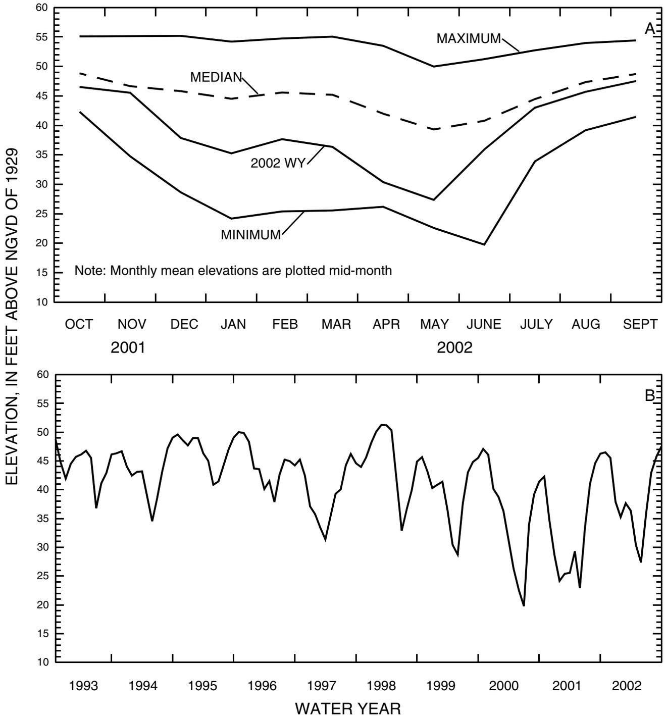
Figure 8.--Marshall deep well near Gardner, Upper Floridan aquifer, (A) 2002 monthly mean elevation compared to the maximum, median, and minimum monthly mean elevation for the period of record, and (B) the monthly mean elevation for the period 1993-2002.
