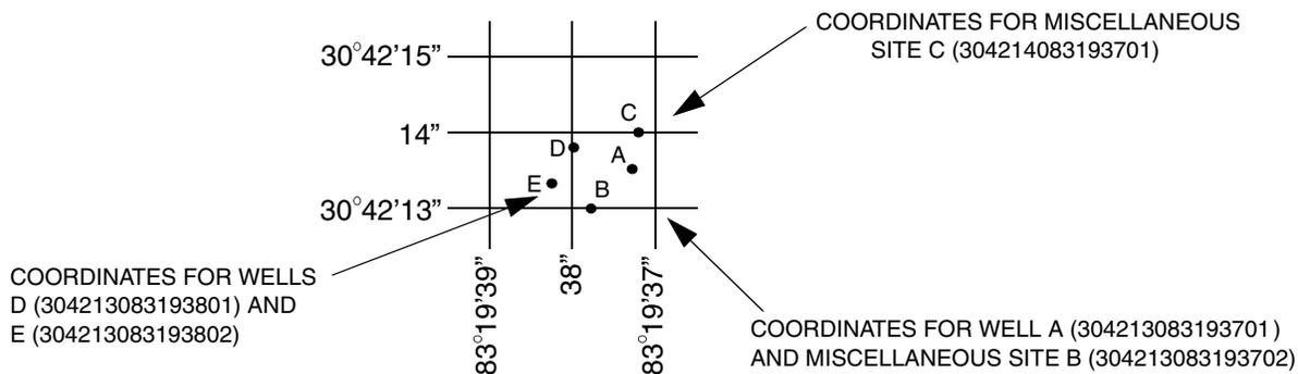
Figure 9.--System for numbering wells and miscellaneous sites.
