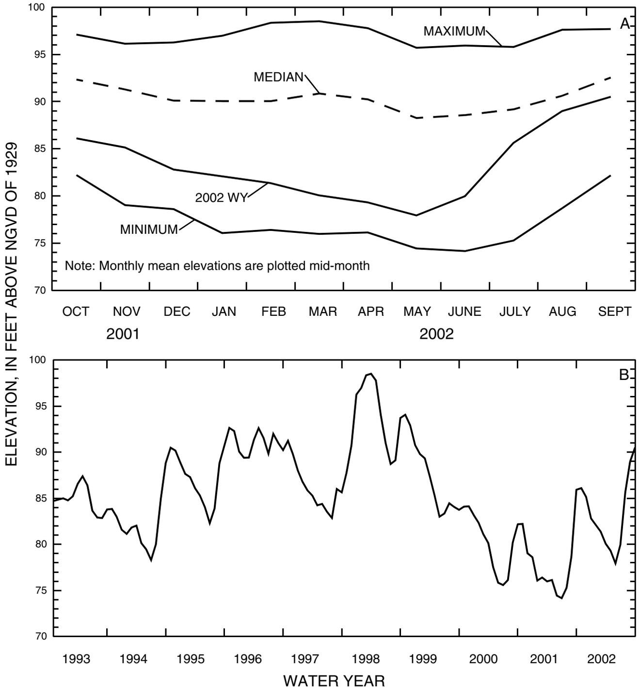
Figure 4.--State Highway 577 well near San Antonio, Upper Floridan aquifer, (A) 2002 monthly mean elevation compared to the maximum, median, and minimum monthly mean elevation for the period of record, and (B) the monthly mean elevation for the period 1993-2002.
