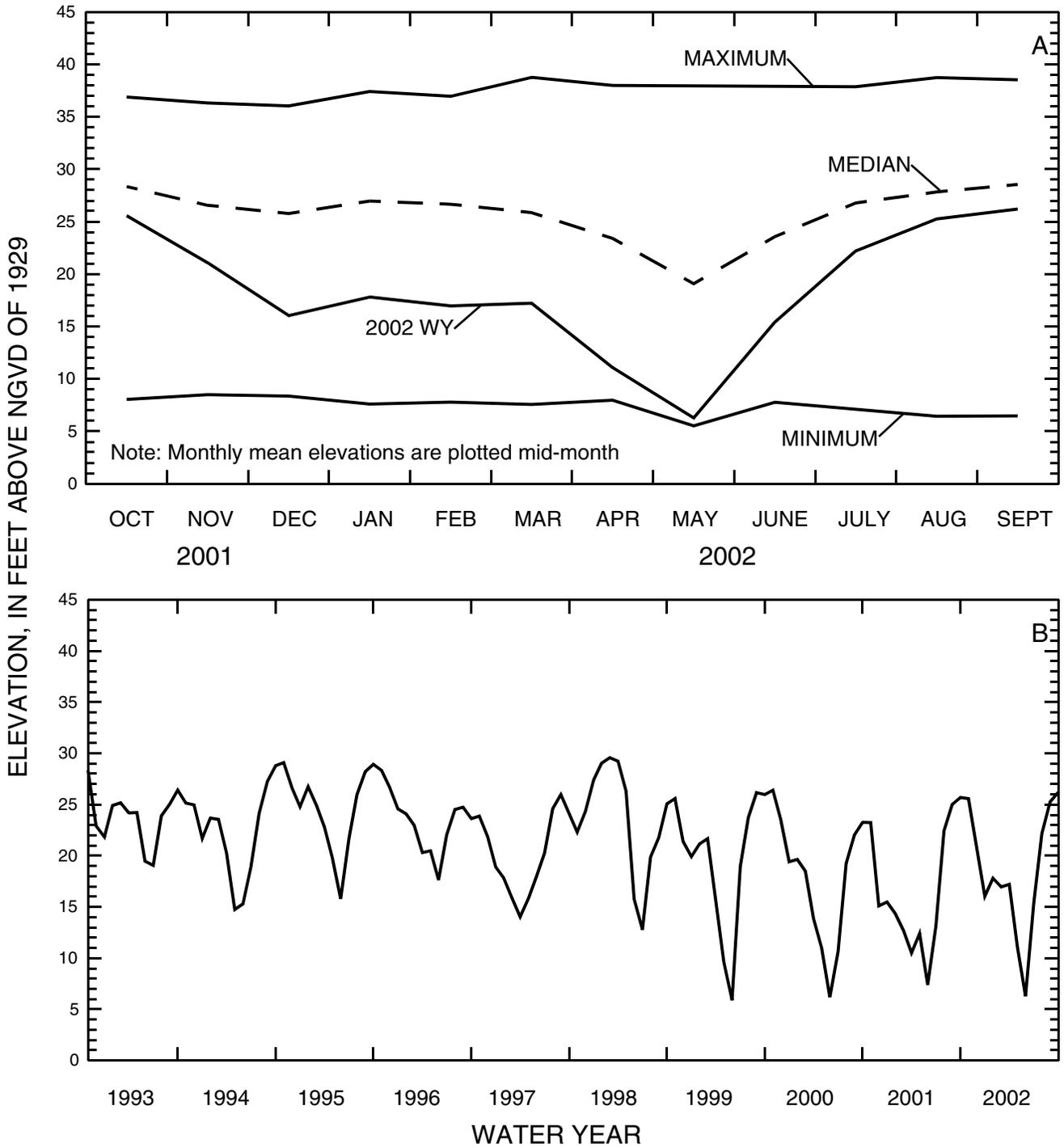
Figure 7.--Sarasota well 9 near Sarasota, Upper Floridan aquifer, (A) 2002 monthly mean elevation compared to the maximum, median, and minimum monthly mean elevation for the period of record, and (B) the monthly mean elevation for the period 1993-2002.
