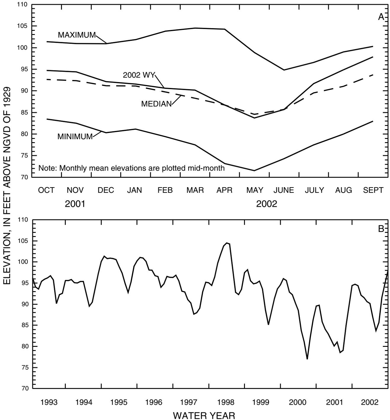
Figure 5.--Sanlon Ranch deep well near Eaton Park, Upper Floridan aquifer, (A) 2002 monthly mean elevation compared to the maximum, median, and minimum monthly mean elevation for the period of record, and (B) the monthly mean elevation for the period 1993-2002
