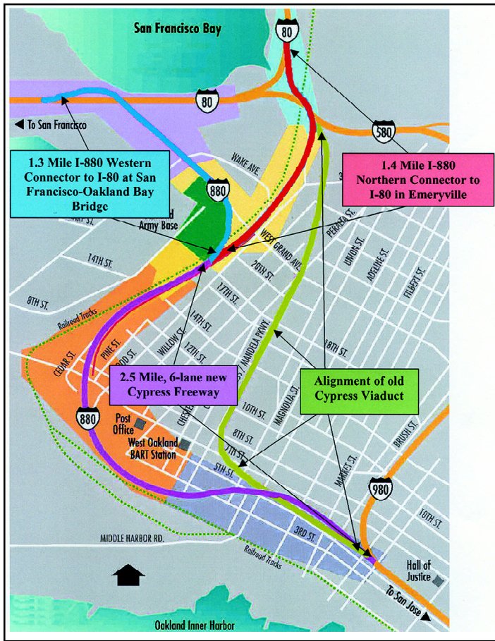
The new Cypress Freeway alignment ran west of the original structure, avoiding most residential areas of West Oakland.
