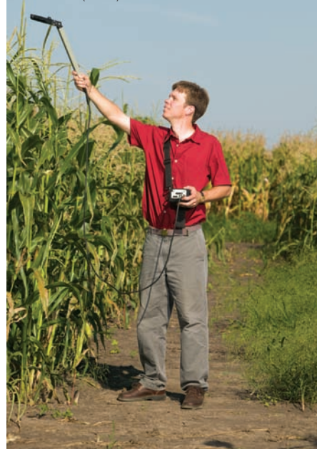
Weed-suppressive traits, such as crop height, leaf area, and growth rate, vary widely among sweet corn hybrids. Ecologist Marty Williams measures solar radiation intercepted by different sweet corn hybrids to determine how canopy structure affects the crop's ability to compete with wild proso millet.
