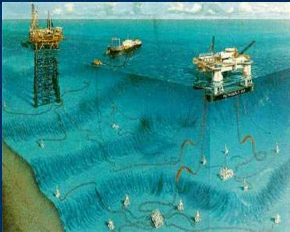
Deep water production systems
