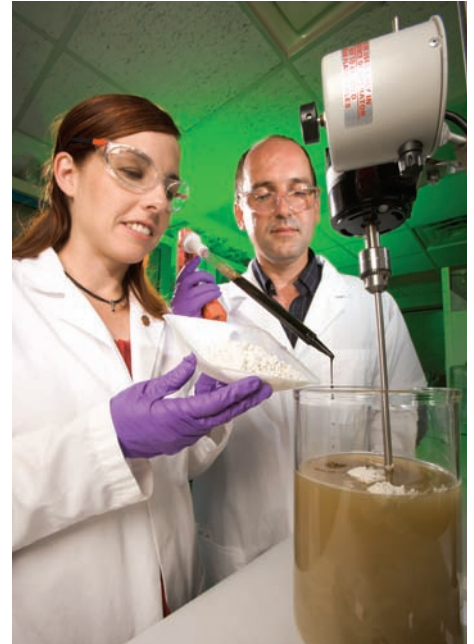
Technician Bridgette Duplantis and chemist Chris Dunlap prepare Paecilomyces fumosoroseus fungal powder and keratin solution for field application. This liquid will turn into a foam when placed in a pressurized foaming machine.
