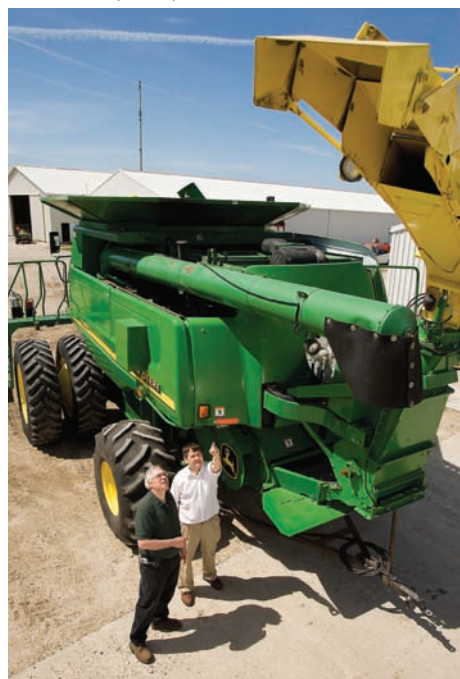
Soil scientist Doug Karlen (left) discusses commercial combine modifications that Stuart Birrell, associate professor at Iowa State University, designed to collect corn stover as a bioenergy feedstock for the REAP (Renewable Energy Assessment Project) cooperative research project.
