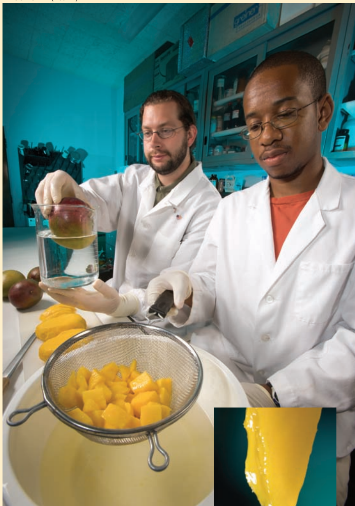
Technician Christopher Ference (above left) sanitizes a whole mango before cutting it into pieces while technician Keith Williamson dips the mango pieces in an edible coating (at right) designed to prolong the cut fruit's shelf life.
