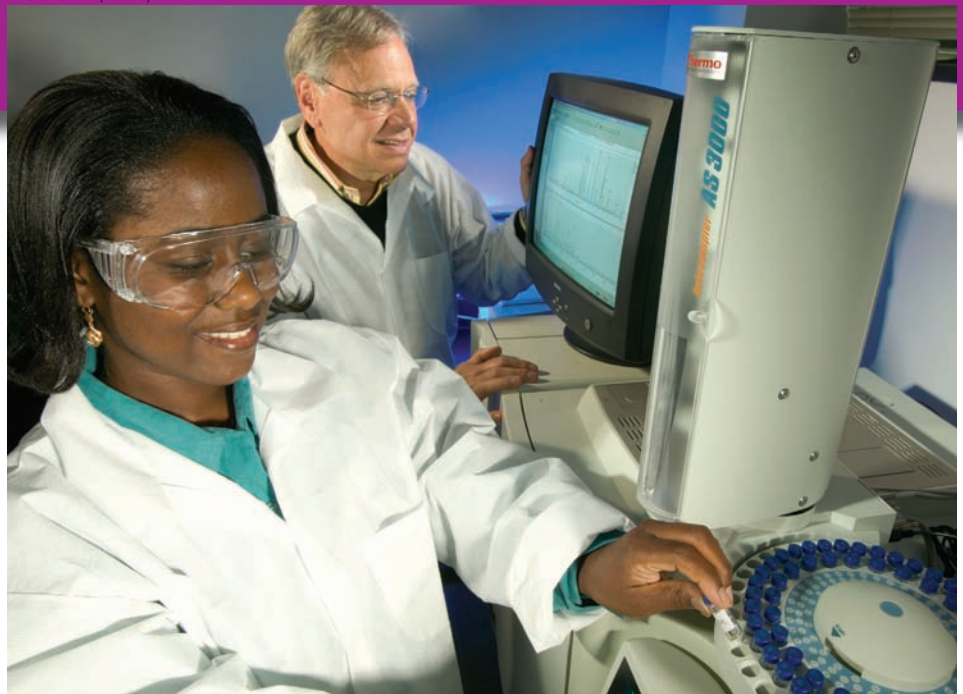
Technician Aisha Abdul-Wakeel places samples into a gas chromatograph while chemist Philip Pfeffer examines mass spectral data to measure the amount of isotopically labeled nitrogen that has been delivered from the mycorrhizal fungus to the host plant.
