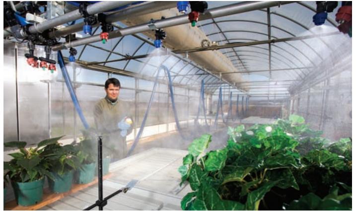
In a greenhouse, postdoctorate researcher Huseyin Güler evaluates new spray nozzles designed and configured to increase efficacy of watering in nursery and other crops.
