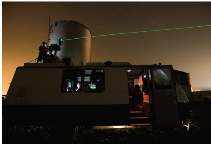
A laser beam from the University of Iowa mobile facility lab is positioned to track the particulate plume from a swine facility.
