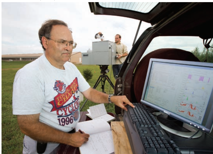
In an air quality study, chemist Richard Pfeifer observes the spectra of gases obtained from an infrared spectrometer unit positioned adjacent to a swine facility.
