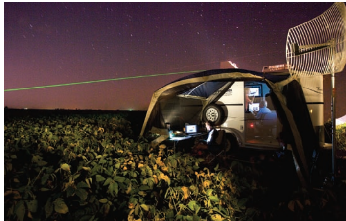
A LiDAR laser from the Space Dynamics Laboratory mobile system is seen tracking across an Iowa landscape to measure the particulate plume at night.
