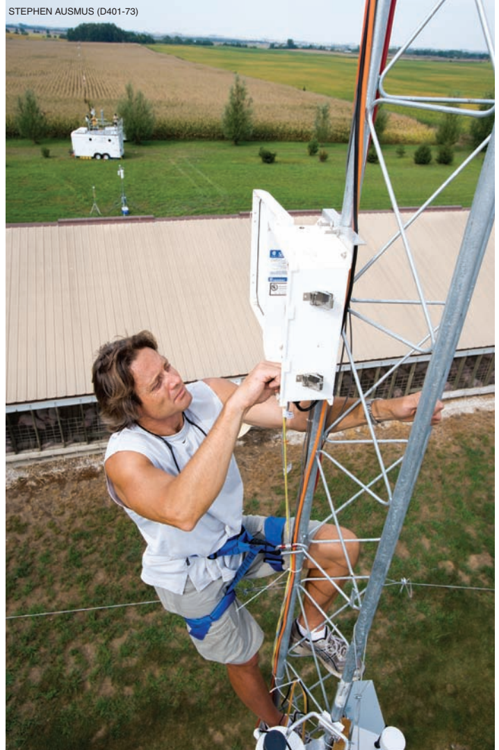
In a study to document plume characteristics with LiDAR measurements, soil scientist John Prueger climbs a 30-meter tower positioned between swine production buildings to inspect air-sampling equipment.
